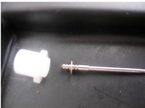
Now you need to remove the fixed washer. You can do this by using the pliers to pop the washer off. Be sure not to bend the needle, it is easy done and would make it unusable! The washer now needs replacing onto the needle, but now, place it onto the middle groove. See photo
