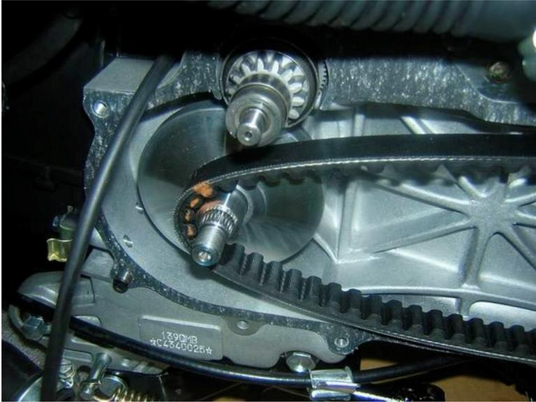
Once removed you should be left with the front drive pulley looking like this...
