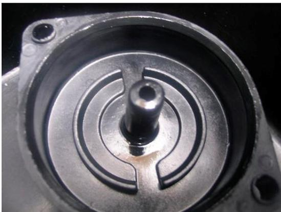
On the under side of the black cap there may be a brass screw in the centre, if there is remove it. Now place the big spring in and replace the cap.
