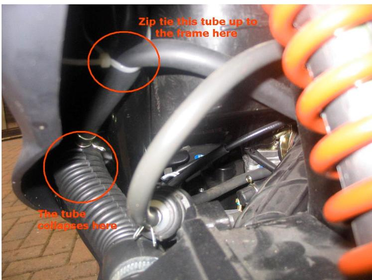
You can do this a couple of ways. You could place a plastic tube inside the hose to stop it collapsing or you could 'zip tie' the smaller tube to the frame, again stopping it from collapsing. I tied the small tube to the frame, see photo.
