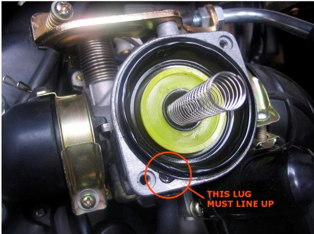
Now you need to put everything back together. Replace the black rubber seal and tube into the carb first. When you do you will need to ensure that the small lug is lined up with the recess in the carb top, and that the seal is seated correctly. (See Photo Below)
